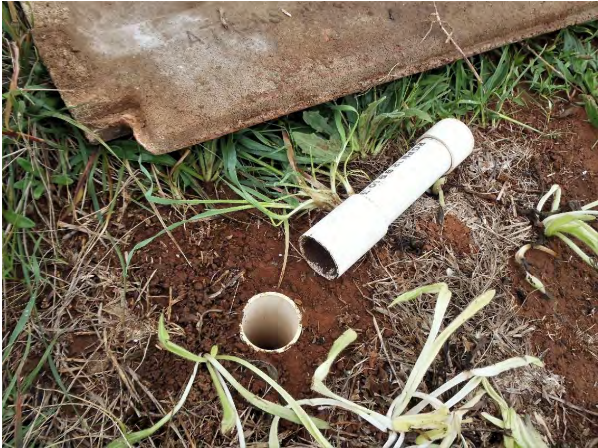
Photograph 1. Artificial burrow (tube) under tile, insert removed. Insert has drainage hole at base and a roughened lining which allows animals to enter and leave.
