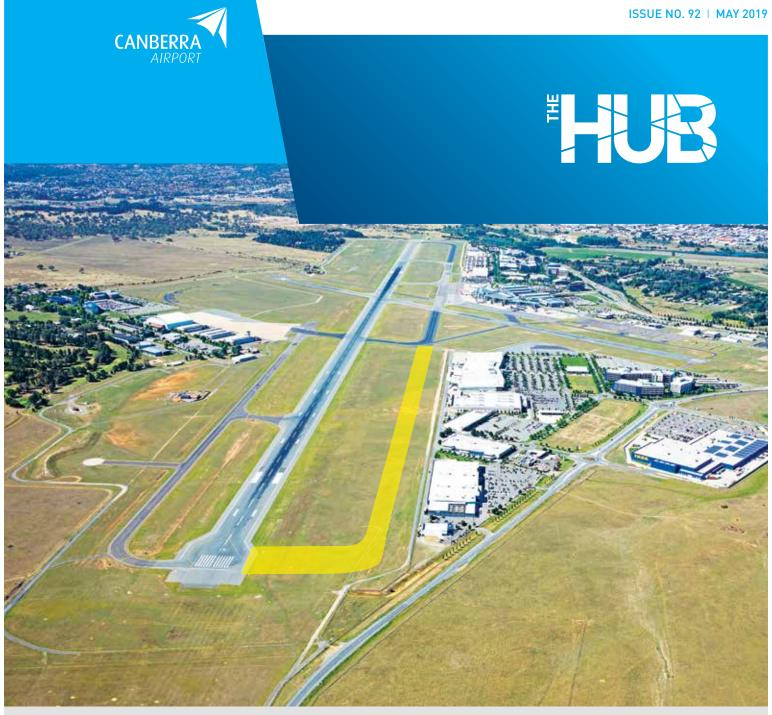
WORK HAS BEGUN TO LENGTHEN TAXIWAY BRAVO AND HELP TAKE THE PRESSURE OFF OF TAXIWAY ALPHA, WHICH WAS BUILT JUST AFTER WWII.
