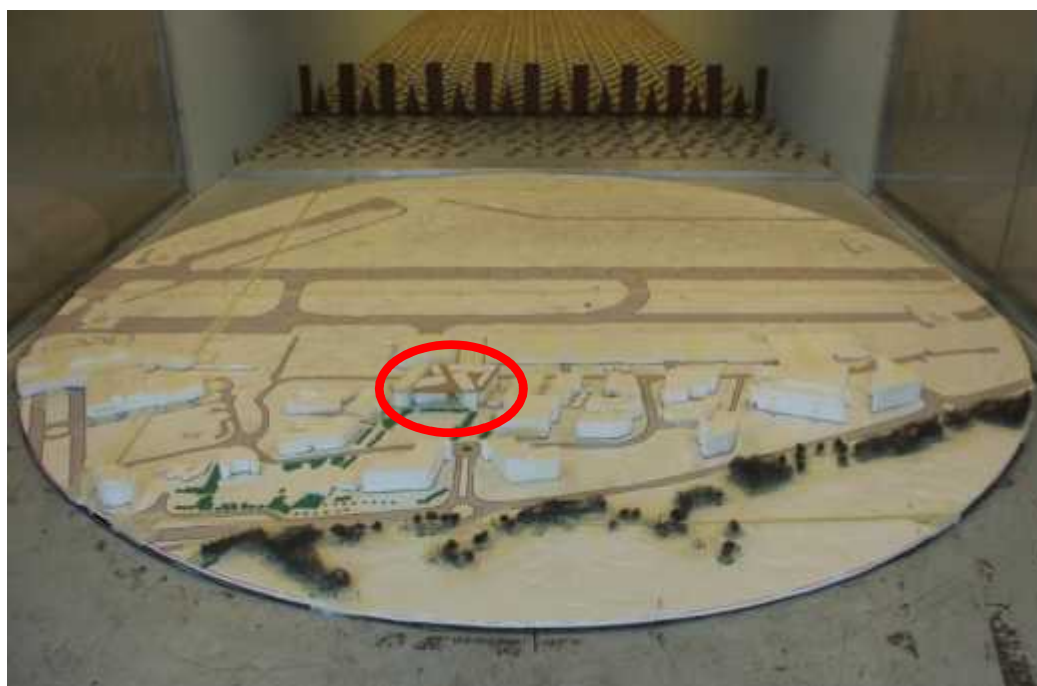
Figure Seven: Photograph of the Model in the Wind Tunnel for Runway 17/35 (view from West, Existing + Proposed)
