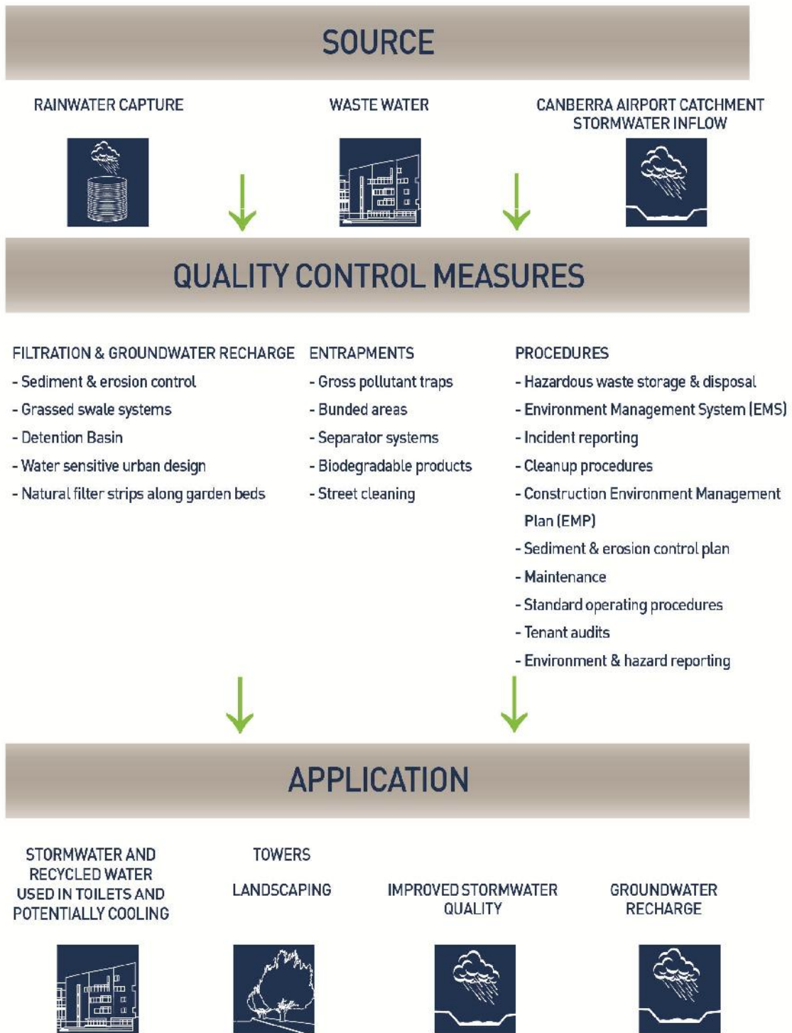
Figure 3.1 - non-potable water flowchart
