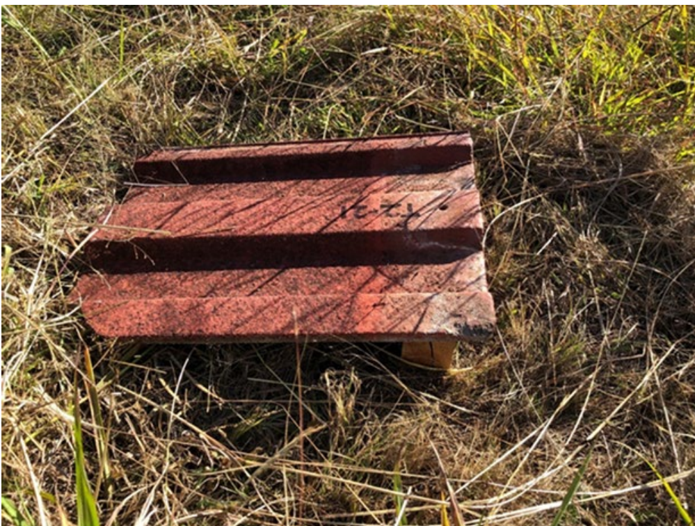
Photo 2.2 Roof Tile Propped at One End on a Thick Wooden Batten
