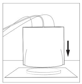
Always use the buffer (part of the packaging) when placing the BuzziBell on the floor or table during installation. This to prevent damage to the felt cover.
