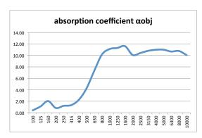
Equivalent sound absorption surface for an individual object in  $\mbox{\em m}^2$
