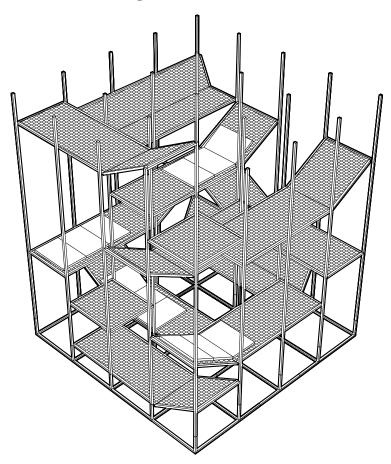
Powder coated metal frame in Fluo Yellow (RAL 1016) Mesh Galvanized
