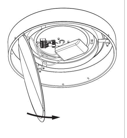
! Make sure wires are not pinched in-between during this step!
