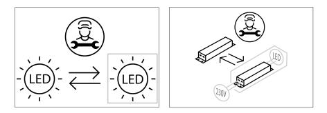
A The light source of this luminaire is not replaceable. When the light source reaches its end of life the whole luminaire shall be replaced.
