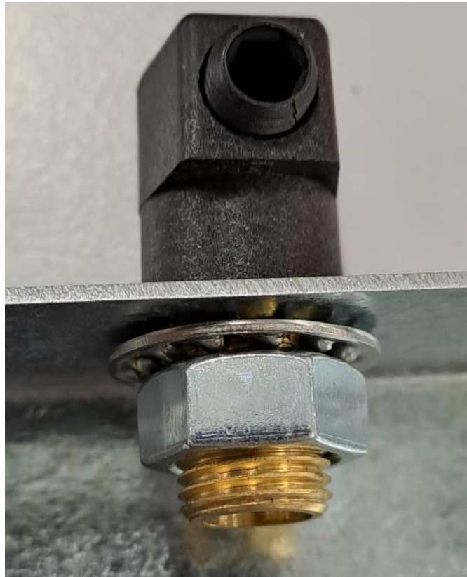
Cord anchorage replacement.
