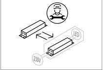
**A** The light source of this luminaire is not replaceable. When the light source reaches its end of life the whole luminaire shall be replaced.
