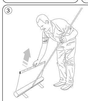
Leaning the pole backwards, extend the top rail with graphic and attach the fixing at the top of the pole.
