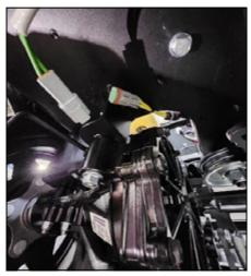
2. Use the strap wrench on the drive pulley of the engine to prevent the engine from turning while removing the bolt.
