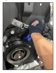
3. Use the Ratchet and the 5/8" socket to remove the crank bolt, pointed out below, then slide the clutch off the crankshaft.
