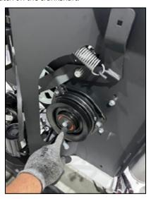
4. Slide the new clutch onto the crankshaft, ensuring the keyway is lined up properly, and the clutch anti-rotate pin is properly engaged as shown below.
