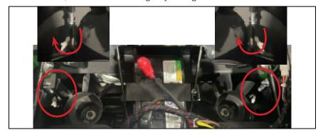
• **IF MACHINE MOVES BACKWARDS** in the neutral position, loosen upper and lower jam nuts. (Note: Lower jam nut is reverse thread) Then, shorten the drive linkages by turning the rod clockwise.
