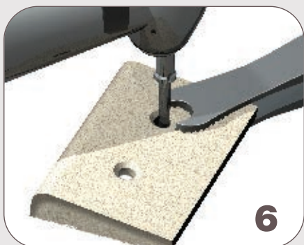
Use the Contra Angle Two-Step Countersink Bur (45440203 F p.26) to make the screw access hole through the graft to the 1.6mm diameter portion of the block graft. (See step 7 for a detailed view).
