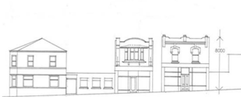
Figure HOB-S2.2 - Building Form: Height, example of buildings of appropriate height
