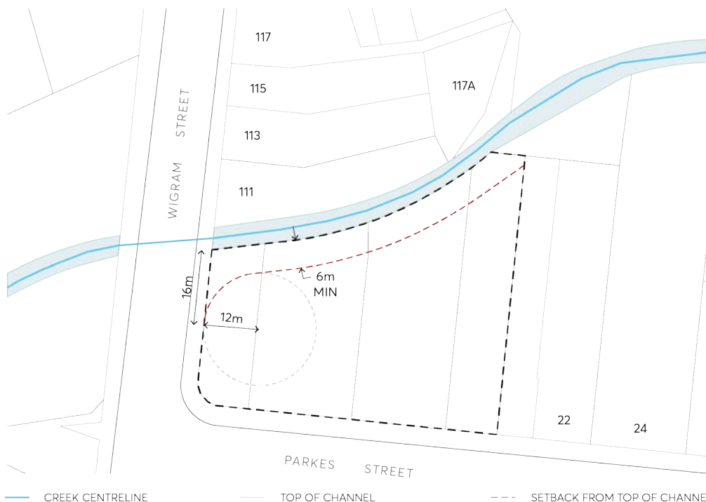
Figure 9.10.8.2 – Required floodway setbacks
