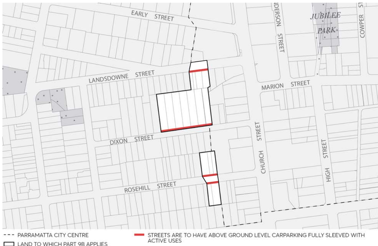
Figure 9B.4.3 – Above Ground Carparking Frontage Treatments
