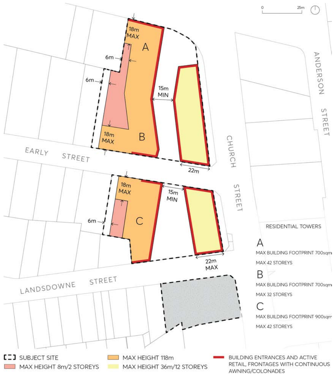
Figure 9.10.2.3 – Building Form Control Plan
