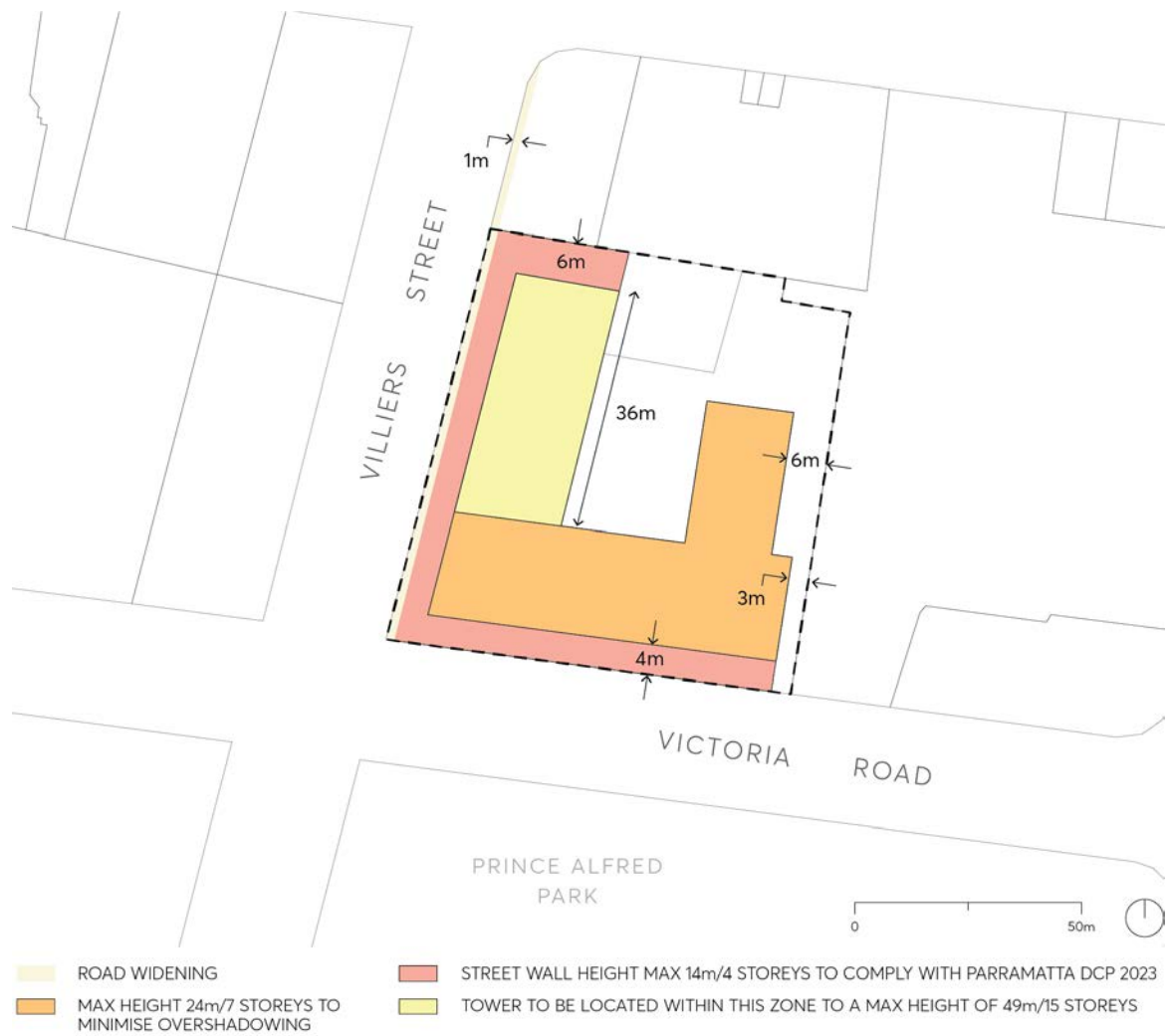
Figure 9.10.19.1 – Built Form Design Controls – Heights and Setbacks
