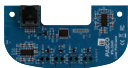
The Line Follower enables the PASCObot to detect and respond to custom line paths that students create using the included tape.
