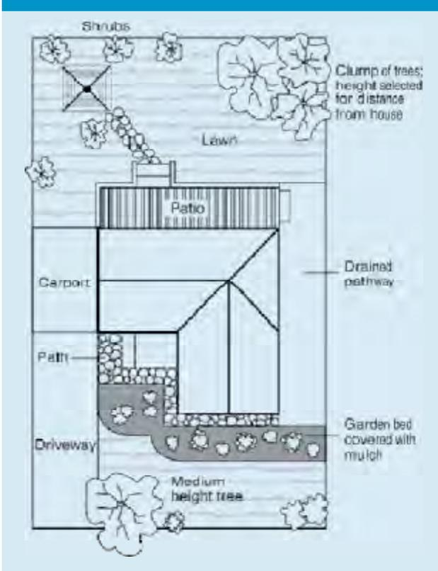
should extend outwards a minimum of 900 mm (more in highly reactive soil) and should have a minimum fall away from the building of 1:60. The finished paving should be no less than 100 mm below brick vent bases.
