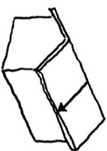
Skillion roof angles between 10-15 degrees
