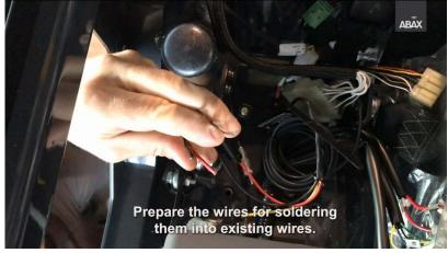
Use a solder iron or an appropriate connecting tool to connect the red wire to a permanent feed, black to ground and yellow to an ignition source. Where appropriate, cover with heat shrink tubing to prevent short-circuiting.
