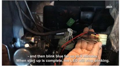
Secure and cable tie any loose wires. Ensure that they will not get trapped or interfere with hot or moving parts.
