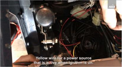
Prepare the ABAX wires for soldering.
