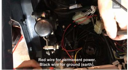
Use the multimeter to verify that the 12V/24V power source is permanent and that the ignition feed switches on/off with the ignition.
