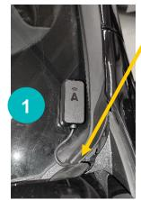
For the best cable routing lift up the rubber.
