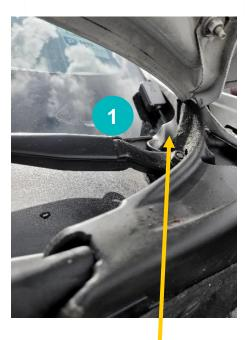
Make sure that the cable goes under the soft material.
