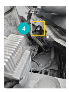
Remarks: The positive connection can be reached by removing the red plastic cover.
