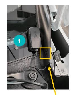
Make sure that the cable goes between the soft material. Loosen the plastic screw.
