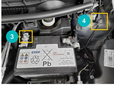
Remarks: The positive connection can be reached by removing the black plastic cover.
