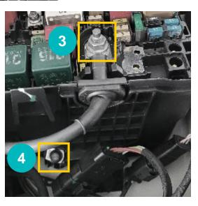
Remarks: The positive connection can be reached by removing the black plastic cover over the fuse box. Push the red wire between the rubber and the housing. Make sure that the cap is replaced correctly.
