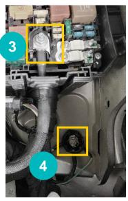
Remarks: The positive connection can be reached by removing the black plastic cover over the fuse box. Push the red wire between the rubber and the housing. Make sure that the cap is replaced correctly.
