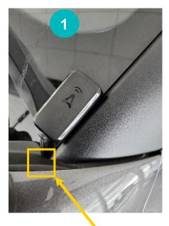
Make sure that the cable goes under the soft material. The rubber part can be easily removed.
