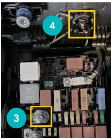
Remarks: The positive connection can be reached by removing the black plastic cover over the fuse box. Push the red wire between the rubber and the housing. Make sure that the cap is replaced correctly.
