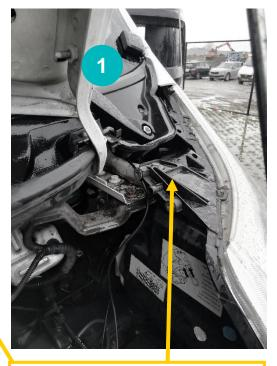
For the best cable routing, remove the plastic panel.
