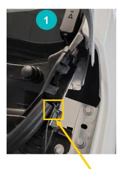
Make sure that the cable goes under the soft material. The rubber part can be easily removed.
