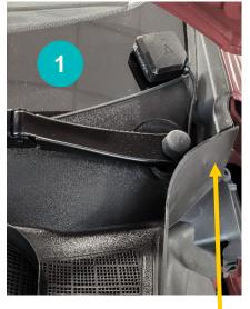
Make sure that the cable goes between the soft material.
