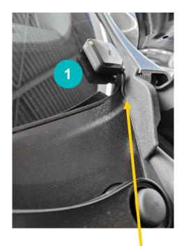
Make sure that the cable goes between the soft material.
