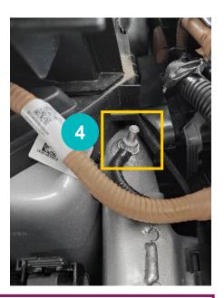
Remarks: The positive connection can be reached by removing the black plastic cap. This is secured with a tie wrap. Make sure that the cap is correctly replaced and secured.
