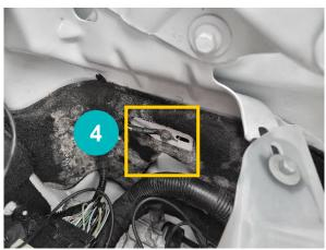
Remarks: The positive connection can be reached by removing the black plastic cover over the fuse box. Make sure that the cap is replaced correctly.
