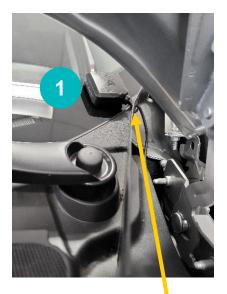
Make sure that the cable goes between the soft material.
