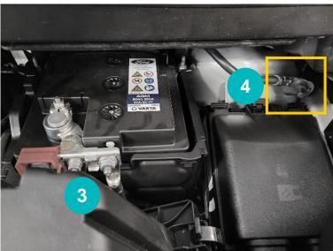
Remarks: The positive connection can be reached by removing the black plastic cover over the battery. Make sure that the cap is replaced correctly.
