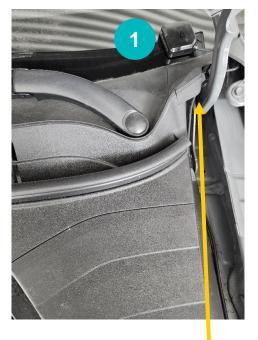
Make sure that the cable goes over the hinge.
