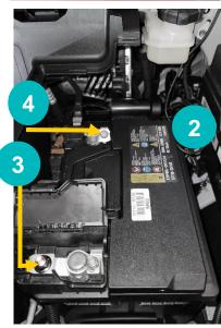
Remarks: To access the battery, remove the black plastic cover. Make sure that the plastic cover is put back correctly.
