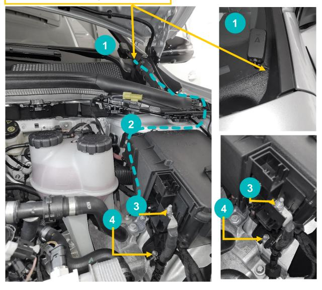
Remarks: To access the +12V connection, remove the black plastic cover. Make sure that the plastic cover is put back correctly.
