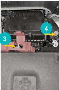
Remarks: To access the positive connection, lift up the red plastic cover. Make sure that the plastic cover is put back correctly.
