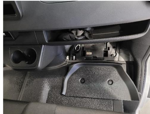
To access the positive and negative connection, lift up the floor cover, and remove the tool holder. Make sure that the everything cover is put back correctly
