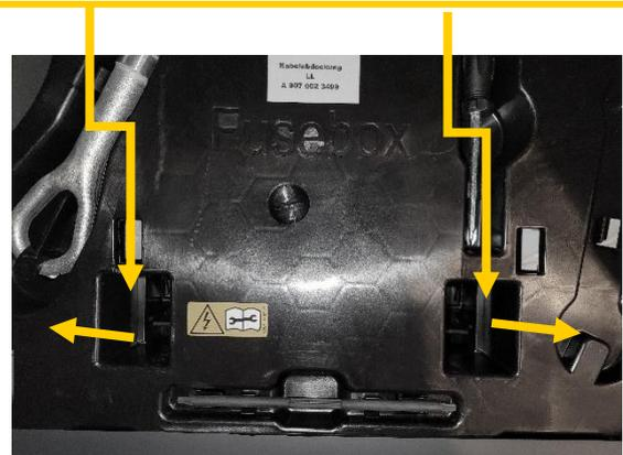
To access the positive connection lift up the fuse box, by loosening the screw.
