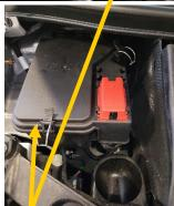
Remarks: To access the positive connection, remove the black plastic cover. Make sure that the plastic cover is put back correctly.
