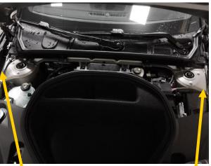
remove the 4 plastic clips by pressing in the middle
