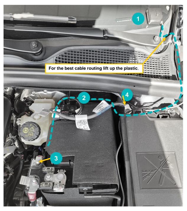
Remarks: To access the +12V connection, remove the plastic red cover. Make sure that the plastic cover is put back correctly.
