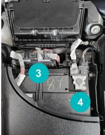
Remarks: To access the +12V connection, remove the plastic red and black cover. Make sure that the plastic cover is put back correctly.
