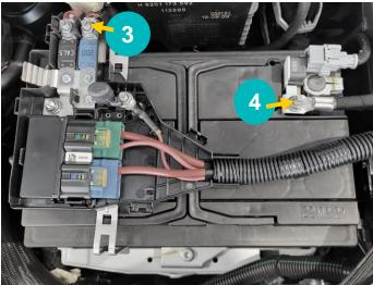
Remarks: To access the +12V connection, remove the plastic red cover. Make sure that the plastic cover is put back correctly.
