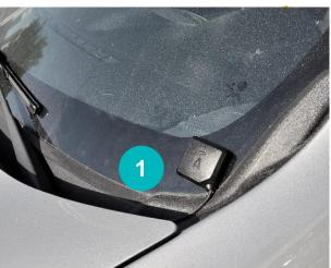
Remarks: To access the +12V connection, remove the plastic red cover. Make sure that the plastic cover is put back correctly.
