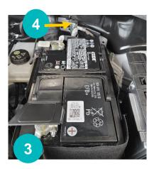
Remarks: To access the +12V connection, remove the small black plastic cover. Make sure that the plastic cover is put back correctly.
