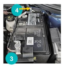
Remarks: To access the +12V connection, remove the small black plastic cover. Make sure that the plastic cover is put back correctly.
