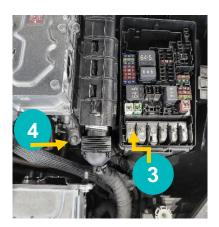
Remarks: To access the +12V connection, remove the black plastic cover. Make sure that the plastic cover is put back correctly.
