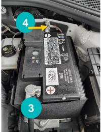
Remarks: To access the +12V connection, remove the small black plastic cover. Make sure that the plastic cover is put back correctly.
