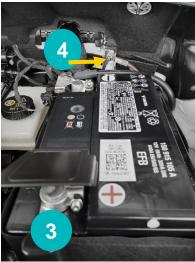
Remarks: To access the +12V connection, remove the small black plastic cover. Make sure that the plastic cover is put back correctly.
